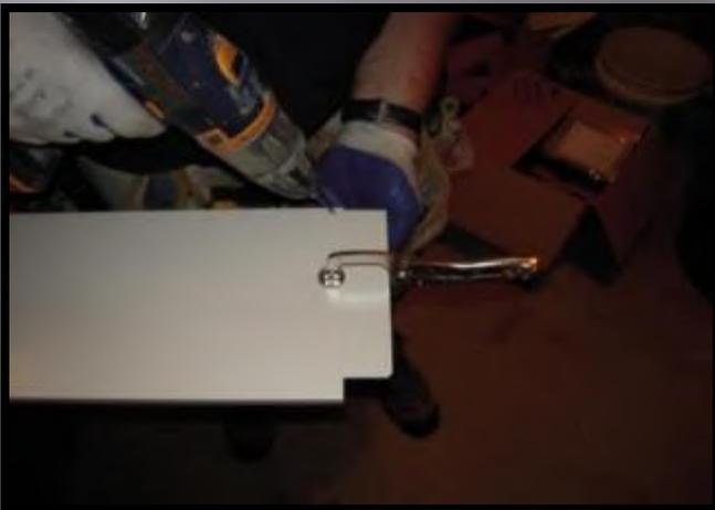
4. APPLY RIVETS, SECURELY ATTACHING COUPLING
